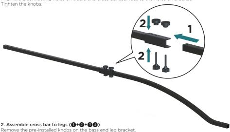
Insert the straight end section of the cross bar into the bracket and align the holes. Insert knobs and tighten.
