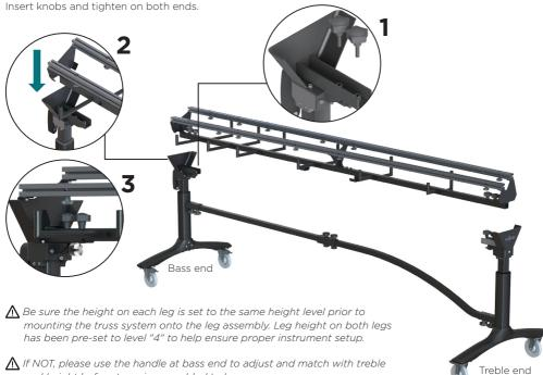
⚠ If NOT, please use the handle at bass end to adjust and match with treble end height before truss is assembled to leg.
