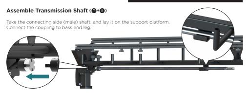
Take the receiving side (female) shaft, and lay it on the other support platform. Push the spring pin on connecting tube, and connect the shafts. Make sure the indicators (a nut on both sides) are aligned.
