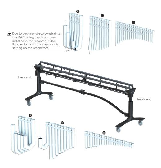
Put the rack on top of the truss, bar posts facing up. Tighten the knobs (4 knobs every section) underneath truss to secure the racks.
